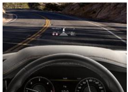
Image displays Windshield Head Up Display
